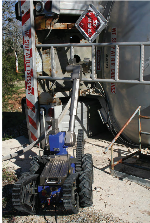
The teleMAX can be equipped with an environment-scanning sensor capable of identifying chemical and biological threats.
