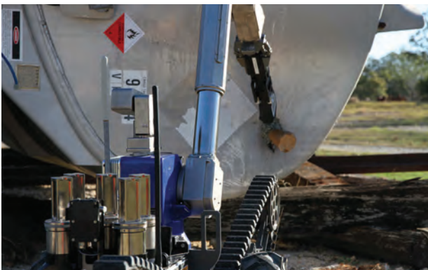
Two chassis-integrated magazines allow the teleMAX to carry more tools and sensors than any other vehicle in its class.
