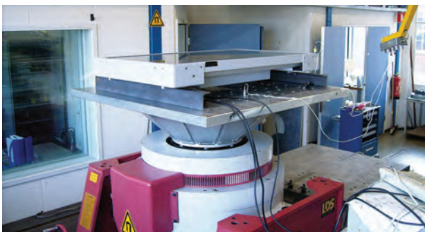
Vibration testing of Conrac's large-screen displays.
