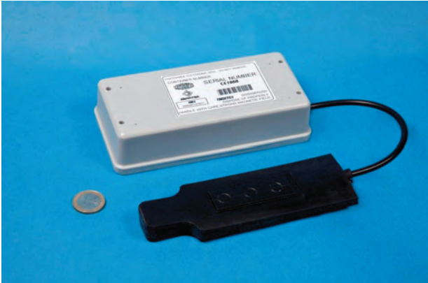
The container-tracking device is designed to be low cost: the device doesn't need to be recovered, and all messages it sends are inclusive of the purchase price. Pictured with a €1 coin to denote scale.
