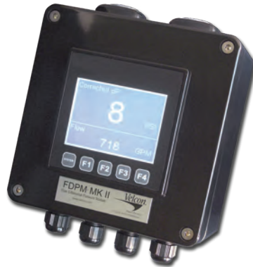
Velcon's FDPM MKII calculates corrected differential pressure across a filter vessel.
